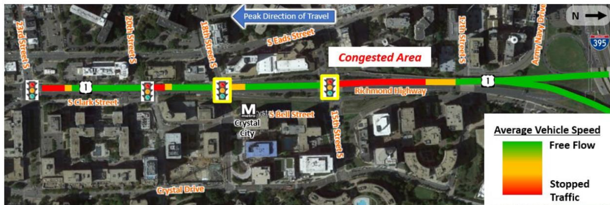
Figure 7-18: Simplified Average Southbound Travel Speeds with Project in Place and 2022 Traffic Volumes
