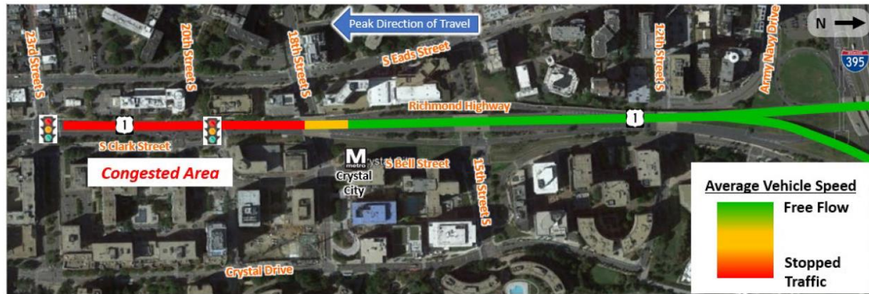
Figure 7-17: Simplified 2022 Average Southbound Vehicle Speeds (Existing Conditions)
