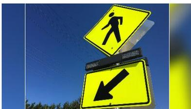
abbreviated RRFB) at a crosswalk near you. An RRFB is a set of high-intensity yellow lights, mounted below the pedestrian warning sign,
